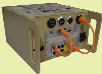
GD2-42MTX - 8 Port Switch, Internal PC, Receiver Unit with internal power supply.
